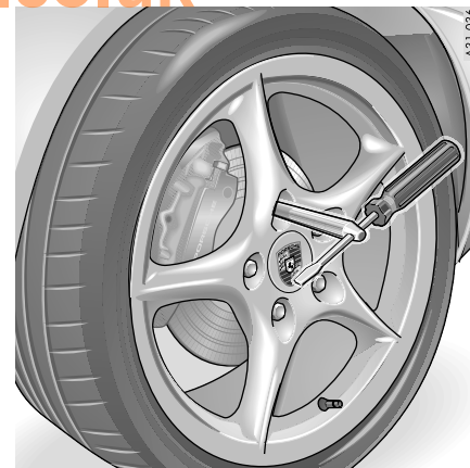
Screwing in assembly aid
